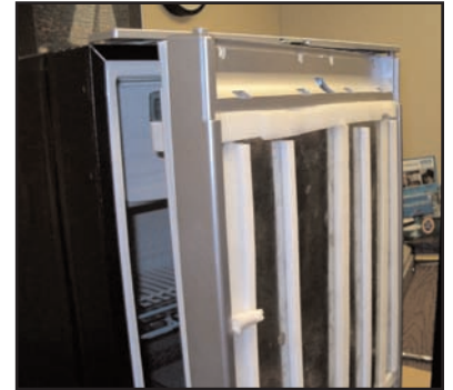
4. Remove the existing face panel, by sliding it up and out of the door surround.
