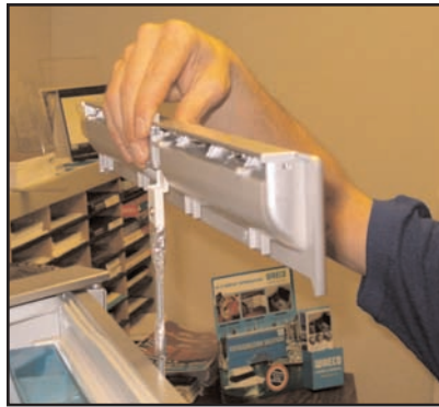
3. Remove the door handle by pulling up until the entire piece is removed.
