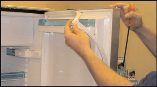
1. Remove rubber gasket from the interior door.
