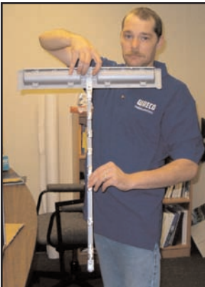
3. Remove the door handle by pulling up until the entire piece is removed.
