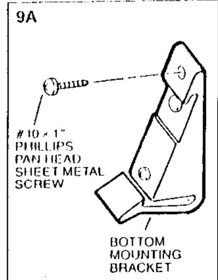
NOTE: The Bottom Mounting Brackets should be mounted to the floorline of solid structural member whenever possible.
