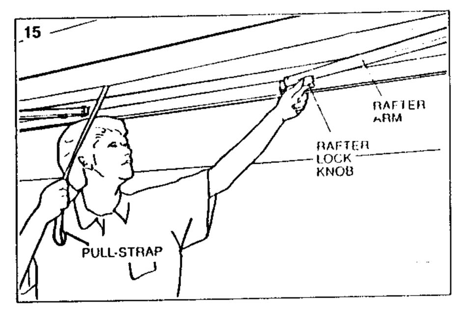
15. While holding Pull-Strap firmly, release Lock Knobs on Rafter Arms and allow awning to roll up. Fig. 15.
