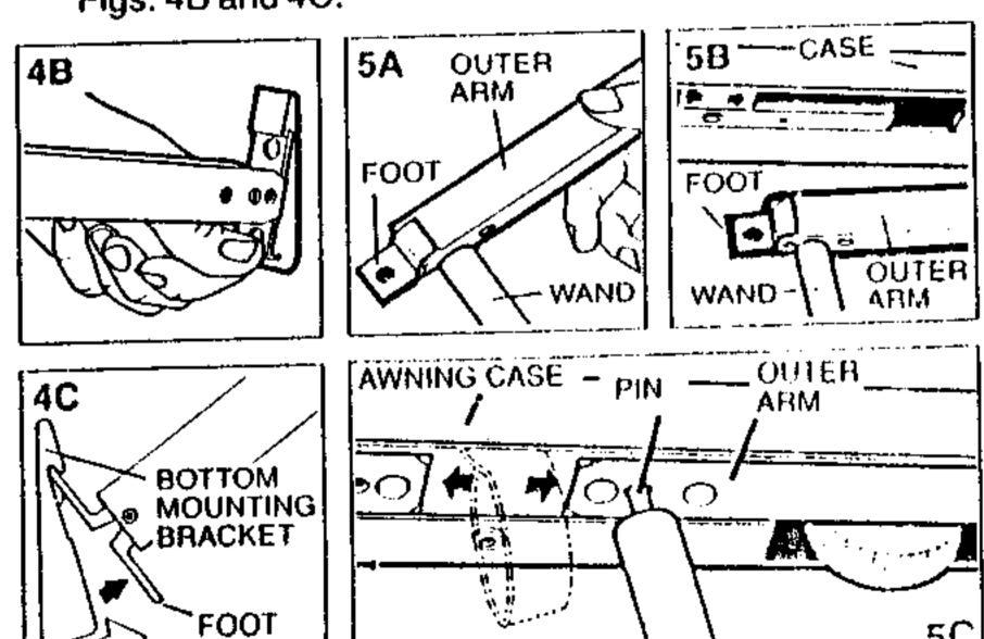
5. Insert Pin at end of Wand through hole in Outer Arm so it aligns Foot for easy storage. Fig. 5A. Swing Arm up to Case. Fig. 5B. Slide Arm and Foot away from center of Case so foot can be inserted into center section of awning Case. Fig. 5C. Repeat for other side.
