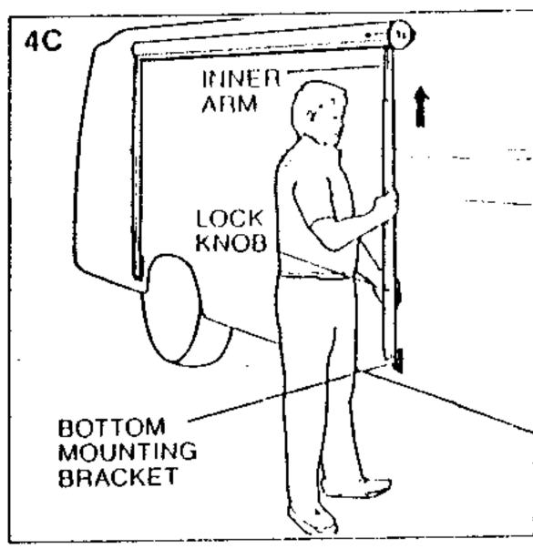
4. A. Set awning into Pivot Position by inserting the awning Foot into the Bottom Mounting Bracket Figs. 4A, 4B and 4C.
