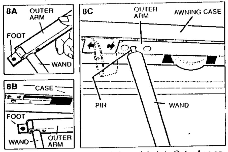
8. Insert Pin at end of Wand, through hole in Outer Arm so it aligns Foot for easy storage. Fig. 8A. Swing Arm up to Case. Fig. 8B. Slide Arm and Foot away from center of Case so Foot can be inserted into center section of awning Case. Fig. 8C. Repeat for other side.
