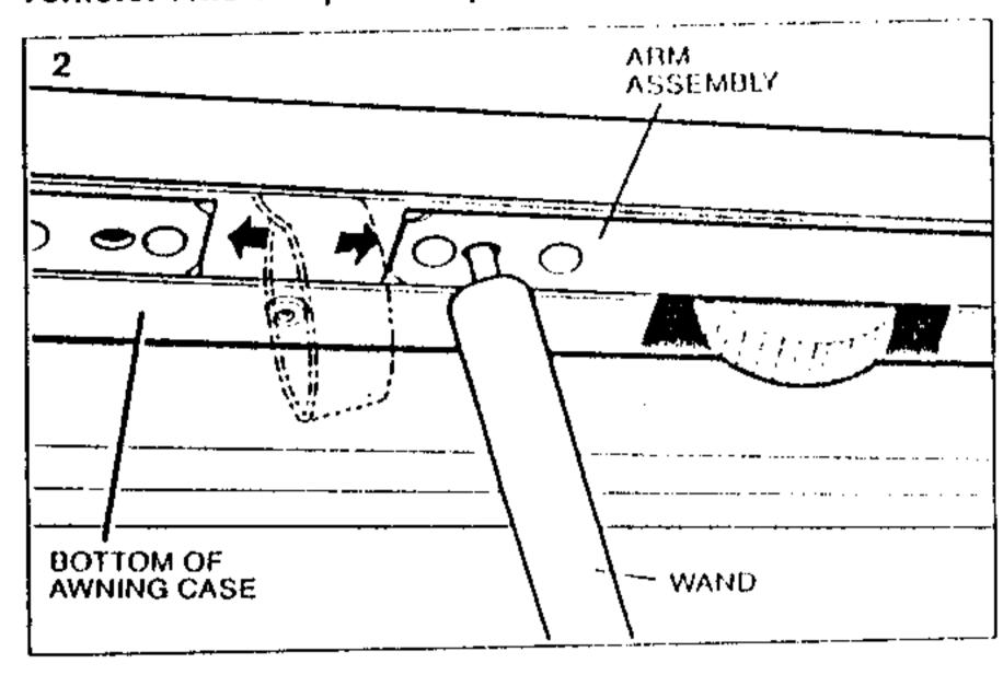
2. Using Wand, open awning Case by inserting Pin on end of Wand into hole in Arm Assembly indicated by arrows on bottom of Case. Fig. 2.
