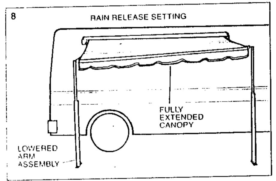
8. Rain Release Setting: To avoid damage to the awning due to rain water collecting on the canopy, simply lower one of the arms enough to let the water drain from that side. Fig. 8.
