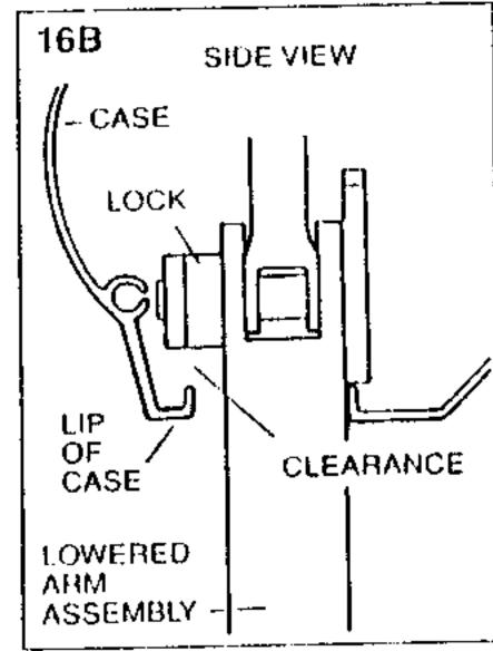
16. For correct installation, Lock in top of awning Arm Assembly must clear top of Case Lip. Figs. 16A and 16B.
