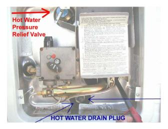
If you store the camper with the hot water tank full of water, the Anode Rod will have a tendency to corrode faster and possibly gunking up the water lines in the camper with a chalky residue. It is always best to flush out the hot water tank periodically to remove any sediment from the bottom of the tank and store the camper with the hot water tank empty.
