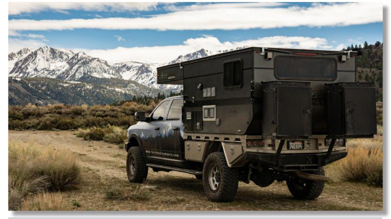
Dry Weight: 1,395 Lbs. Adult Sleeping: 3-4 Height Down (including vent): 60" Extended Interior Height: 6'6" Roof Length: 165" Roof/Wall Framing: Aluminum Floor Length: 94" Exterior Material: Aluminum Body Width: 81" Fresh Water Capacity: 20 Gallons
