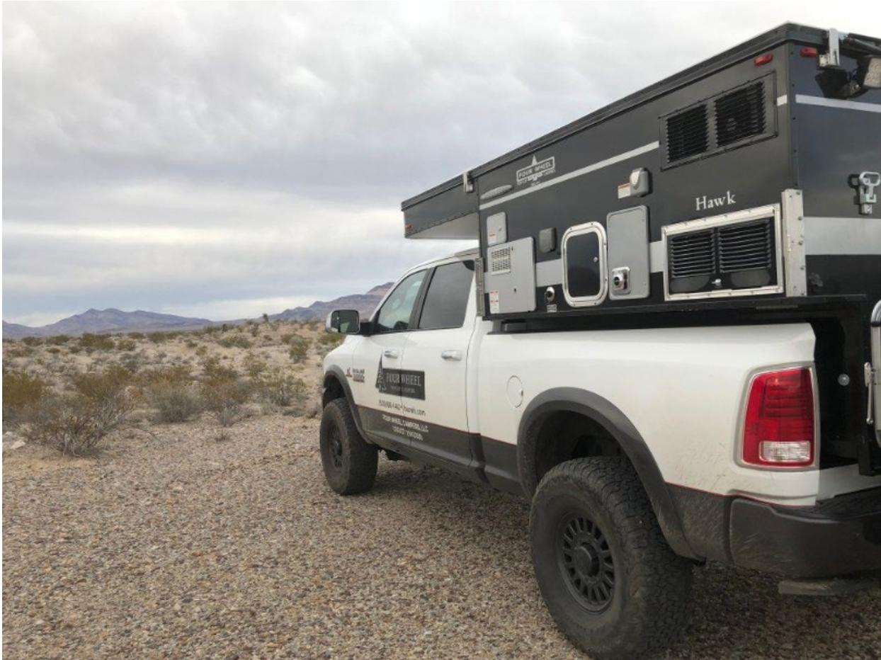
What makes their campers perfect for extreme off-road camping is the durability of the materials used. The frame of the campers is made out of aluminum and the walls are made from a bendable aluminum, allowing it to take a beating from climbing rough terrain and withstand the impact if you bump up against a tree or building.
