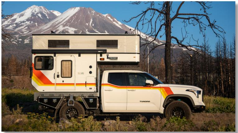
Dry Weight: 1,325 Lbs. Adult Sleeping: 3-4 Height Down (including vent): 62" Extended Interior Height: 6'6" Roof Length: 150" Roof/Wall Framing: Aluminum Floor Length: 80" Exterior Material: Aluminum Body Width: 81" Fresh Water Capacity: 20 Gallons
